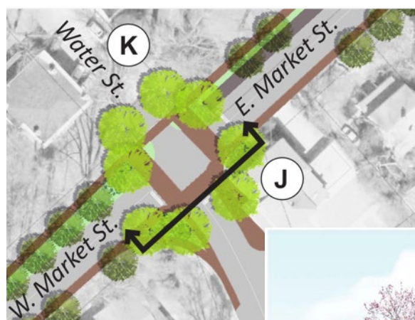
Figure 32 - Proposed crosswalk at the location with the best sight lines for oncoming traffic. The sidewalk shown on the south side of Market east of the crosswalk is a long-term option and would only be built if the roadway is reconstructed and any potential impacts of construction to adjoining historic properties can be addressed.
