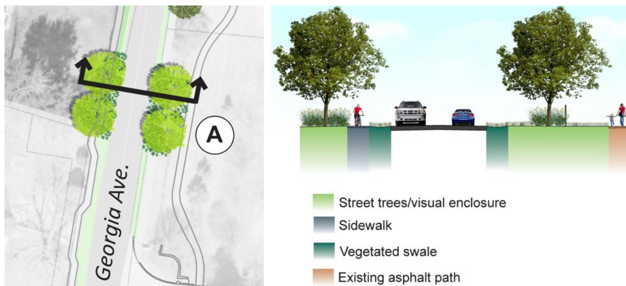
Figure 26 - Georgia Avenue/High Street Gateway illustrating separated shared use path and street trees to begin narrowing the look and feel of the roadway
