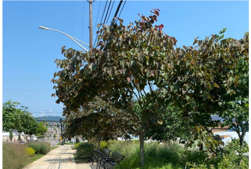
Figure 45 - Small street trees that generally do not grow taller than 20', like this Forest Pansy Redbud, are appropriate for planting under overhead utility lines
