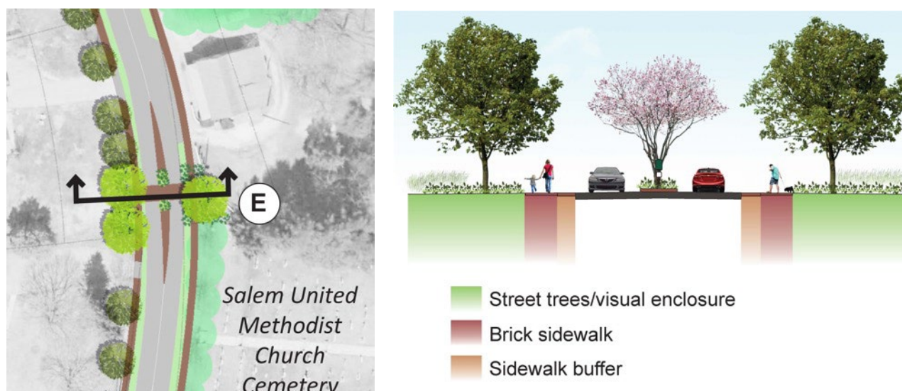
Figure 27 - High Street Transition illustrating the use of a splitter island as a traffic calming measure as well as a refuge island to protect pedestrians in the proposed crosswalk
